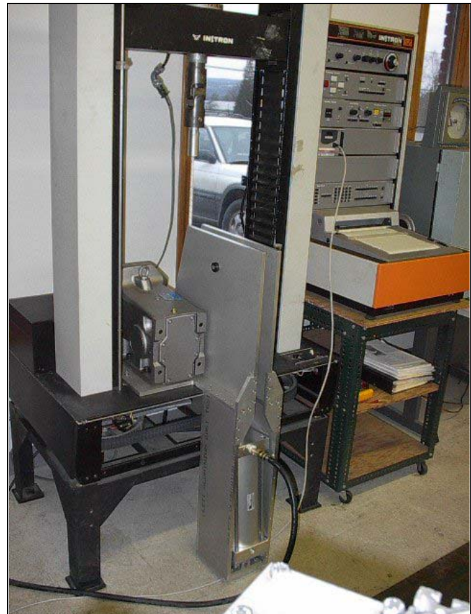
Figure 2: Rope tester mounted on Instron.
