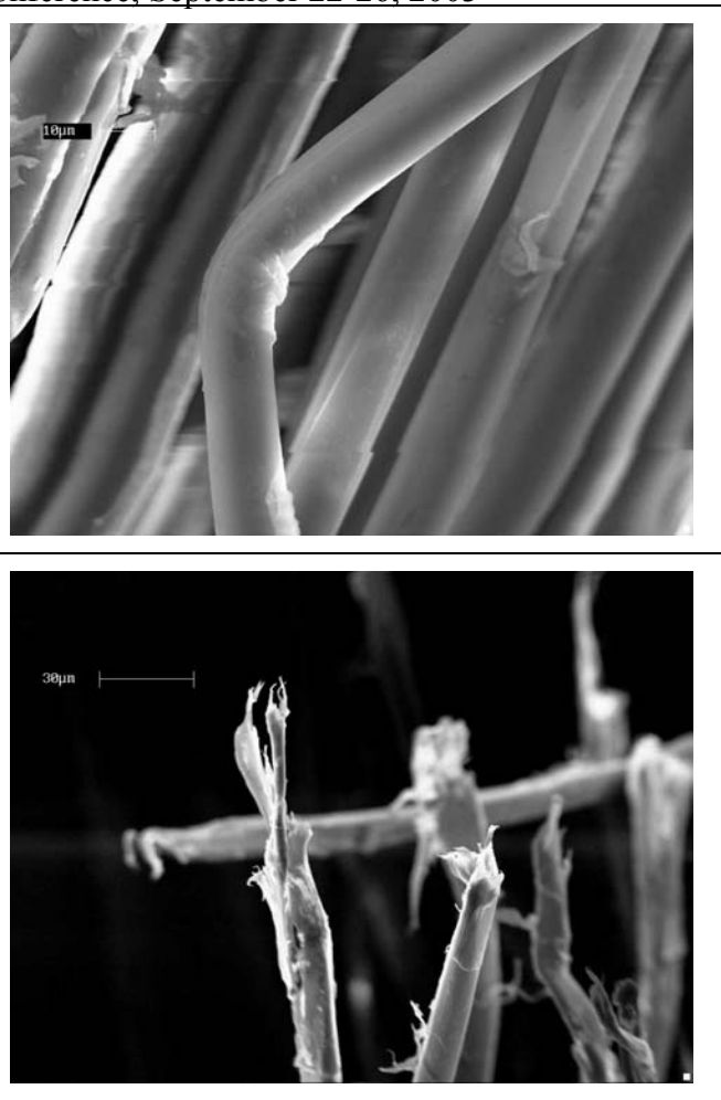
Figure 5: Bent fiber from an outer strand showing compression bands (above) and a fiber from the core, broken in tension, with no sign of fibrillation (below) during bend-over-sheave testing of an unbalanced rope with one end free to rotate.
