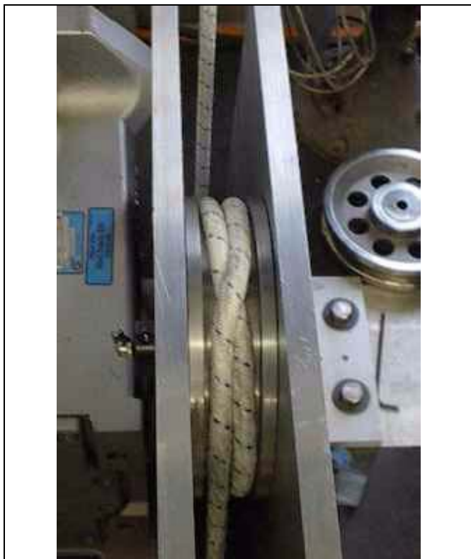
Figure 1: 3/8" Kevlar rope wrapped around a 5.25" diameter drum to simulate poor spooling. An order of magnitude reduction in fatigue life was observed when tested in this configuration.
