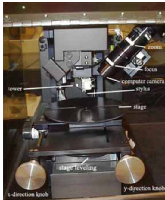
Figure 1. Veeco Dektak 6M Profilometer shown with key features and controls labeled.
