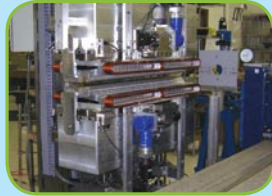
Elliptical Polarization Undulator SRC - USA One Meter PPM Installed
