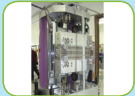
Wiggler Undulator ALBA - Spain One Meter HYBRID Installed
