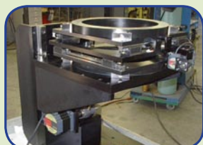
High Precision Upright Cryostat Holder for Spring-8 - Japan
