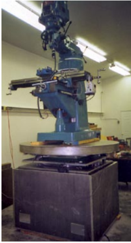
Verifying load capacity with 3000 lb milling machine
